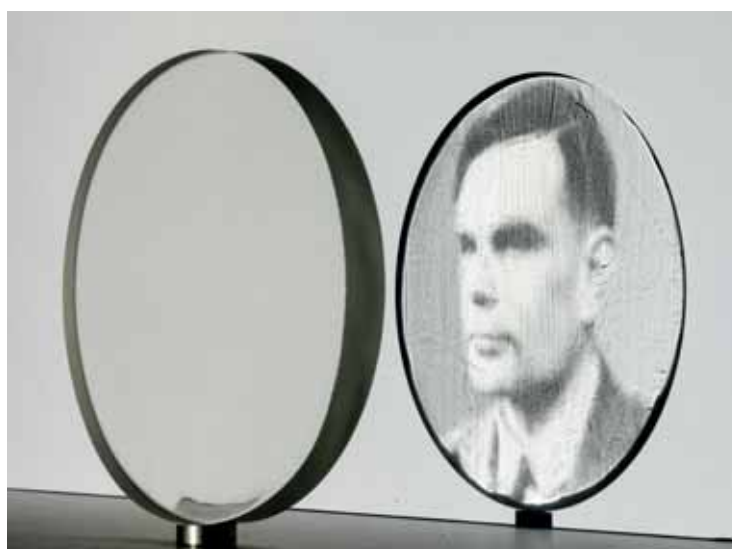
Figure 8 Caustic generated by the sample 3 produced with glass grinding. Insufficient polishing leaves some speckle-noise on the caustic image.
