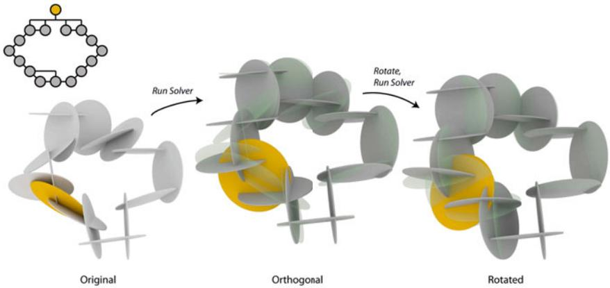
**Fig. 5** A cyclic arrangement of pieces. The graph representing the connections is shown at top-left. Beginning with a non-orthogonal construction at left, we run the optimization solver. Then, as a user edit operation the yellow piece is rotated and the optimization runs again. The transparencies in green illustrate the previous locations of the pieces for comparison. Note that rotating the yellow piece produces changes in many neighboring pieces, and slight changes in far pieces.
