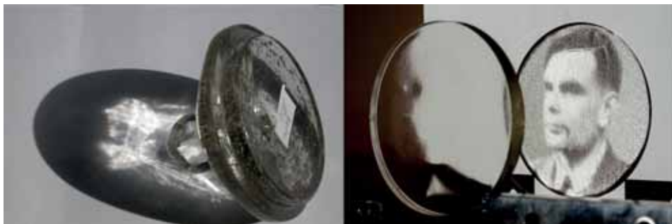
Figure 1 Left: A typical caustic created by a curved glass object appears chaotic and random. Right: Our method creates glass objects that cast controlled caustics by optimization of the glass surface geometry alone. The portrait of Alan Turing emerges from a beam of uniform light that is refracted by the circular glass piece.
