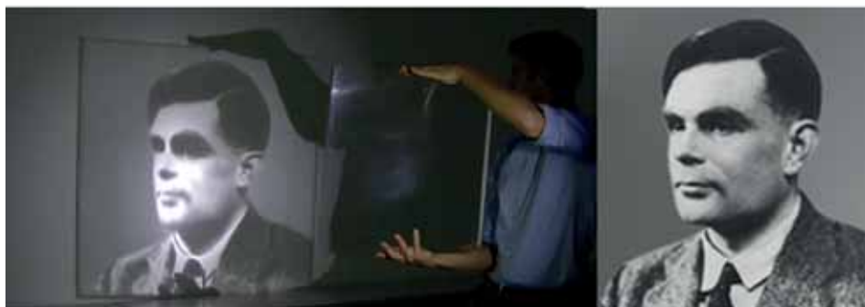
Figure 3 Top: Conceptual sketch of how parallel incoming light is diverted by a glass object to create a desired caustic image. Our algorithm first computes the required surface normals and then integrates the normal field to obtain the curved surface of the glass object. Bottom: A sample of 50cm by 50 cm milled from PMMA and polished by hand to obtain high specularity. When illuminated with uniform light, a caustic image of a portrait of Alan Turing is created (see original photo on the right). Note how the detail of the image is accurately reproduced on the refracted light pattern even though the PMMA plate is just held roughly in position. Even fine-scale detail, such as the weaving of the jacket can be observed.
