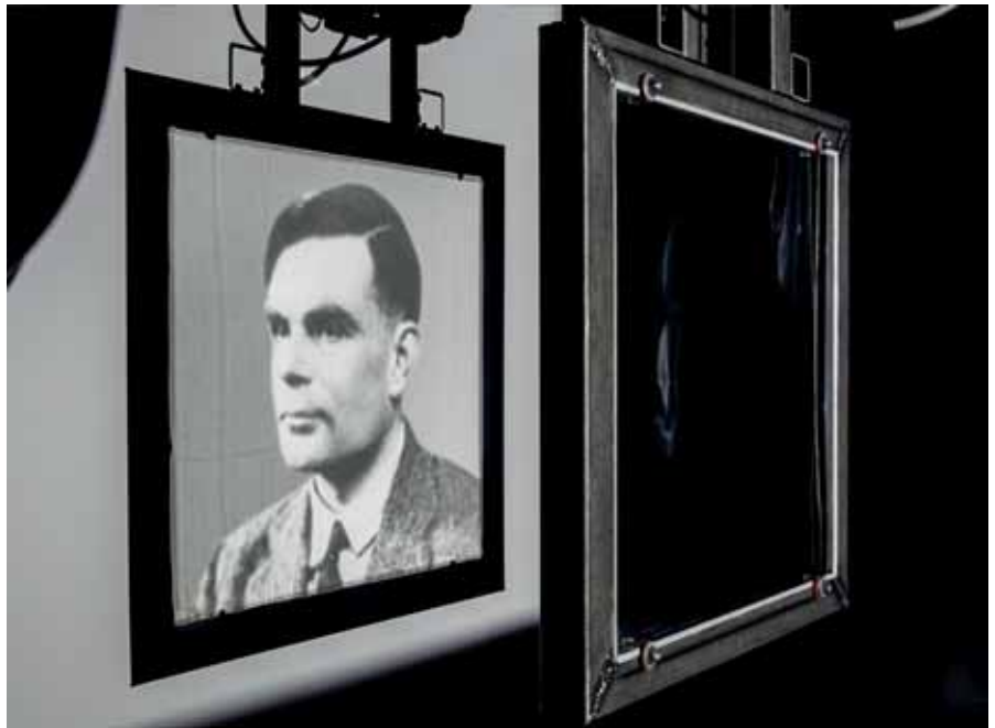
Figure 5 Caustic generated by the milled 500 x 500 mm PMMA Sample 1.
