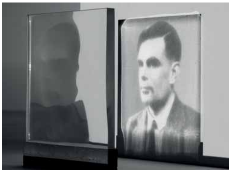
Figure 7 Caustic generated by parallel light through the Sample 2 made of cast Resin.
